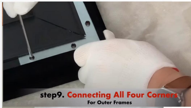
Tighten the small screws on the corner braces. Check the junctures of four corners. If the junctures are big, please adjust the junctures before tightening the screws.
