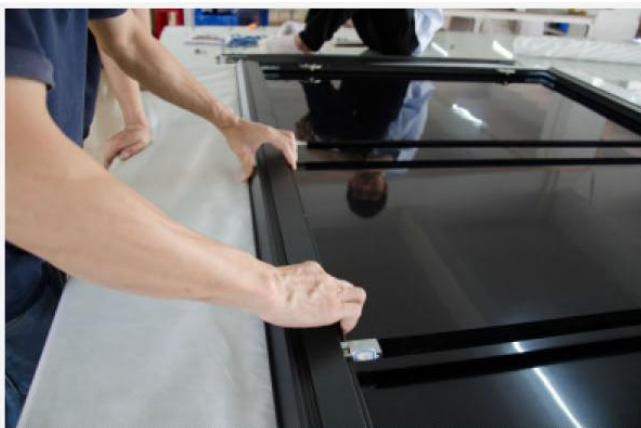
Cover the inner frame with the outer frame. Hold the inner frame and outer frame at the same time, press them together until hear a "click".
