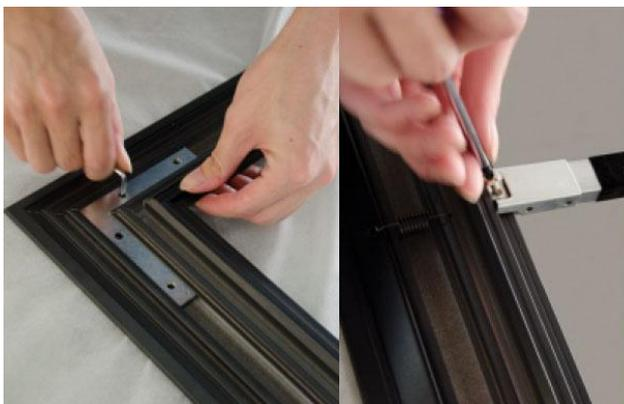
After turning all screws at the four corners, please adjust the junctures of the corners. Hold the frame tightly with one hand and tighten the screws with the other hand. After installing the inner frames, please install the support rods.
