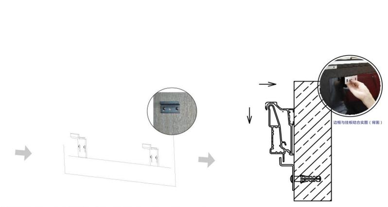
Hang the assembled entire frame screen on the wall mount
