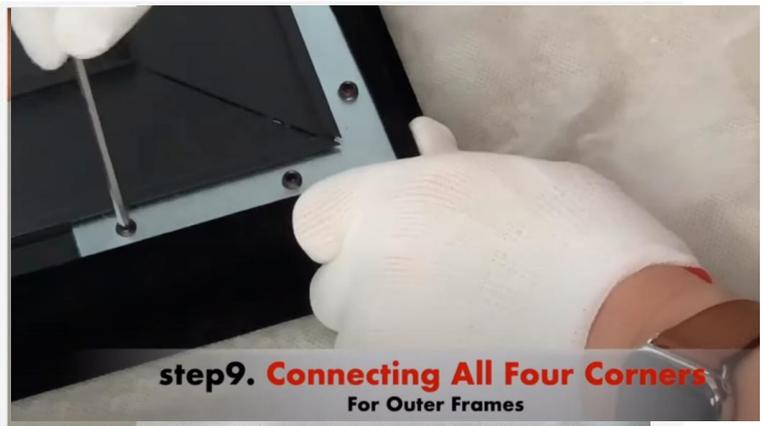
Tighten the small screws on the corner braces. Check the junctures of four corners. If the junctures are big, please adjust the junctures before tightening the screws.
