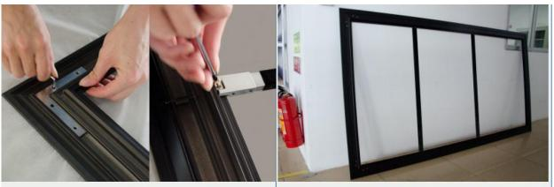
After turning all screws at the four corners, please adjust the junctures of the corners. Hold the frame tightly with one hand and tighten the screws with the other hand. After installing the inner frames, please install the support rods.
