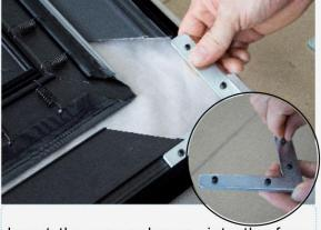
Insert the corner braces into the four corners of the outer frames. Please put the small screws onto the corner braces before inserting them into the frames.
