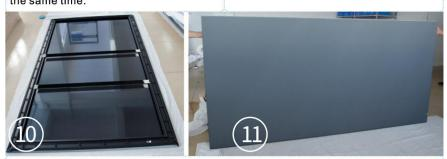
After hooking all the springs, turn over the screen to check whether it is flat. If there is some wrinkles, please adjust the springs and the fabric.
