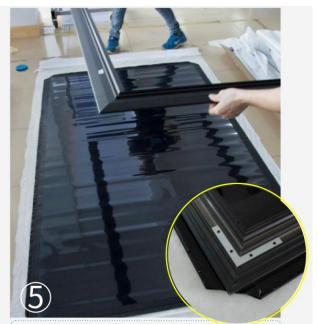
Put the installed inner frame onto the fabric. Note that the four corners must be aligned to the corner cut.
