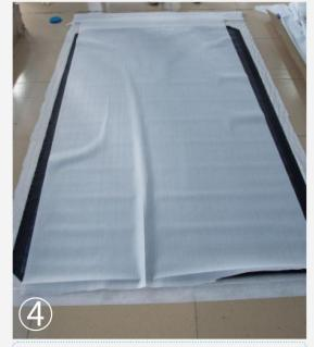
Put the fabric onto the non-woven fabric, with the back side upward.
