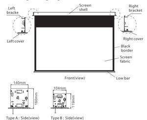
A-Type ceiling cut out dimension: cut out length Lt = Screen Total length – 26mm; cut out width 150mm, height ≥160mm;
